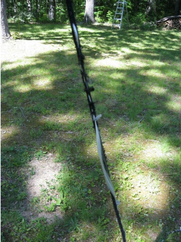
Figure 12. Abrasion-damaged 3/16 inch polyester rope.
