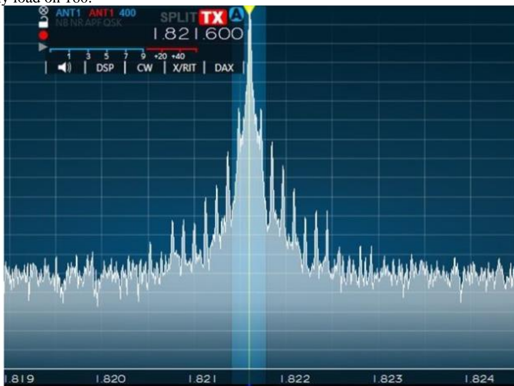
Flex 6600M Band Scope shot of my transmitted signal on 160 M prior to resolving noise problem
