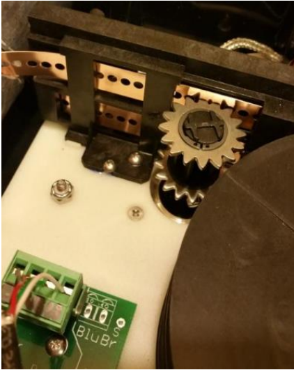
See the perforated beryllium copper strip.
