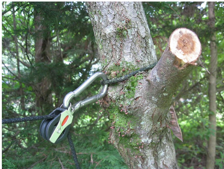
Another pulley attached by a rope tightly girdling the tree.
