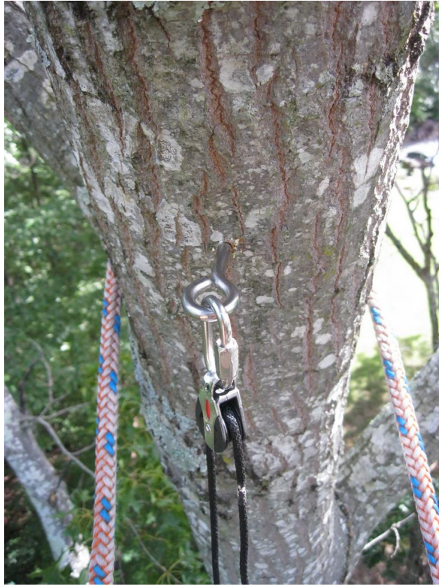
The pulley re-installed on a screw eye.
