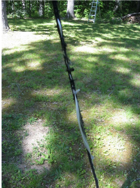
Abrasion-damaged 3/16 inch polyester rope.
