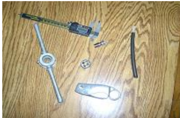
Scrap piece of RG-8 style coax and tools. Precision Calipers, PI-259, Die Holder, 7/16 X 14 Die and a Coax Cutter.
