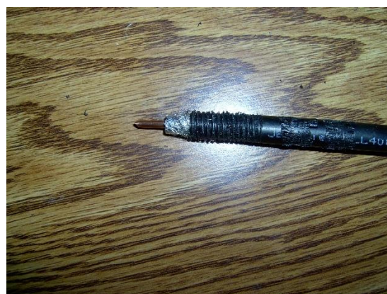
Approximately 1 1/2 inches of Threads Cut
