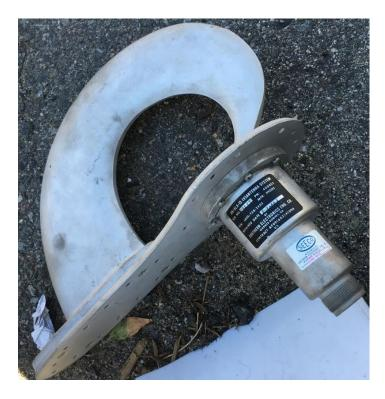
The Scimitar antenna has a long history in both electronic warfare and as a telemetry antenna in the Apollo space program. The inner radius sets the high frequency, and the outer radius sets the low-frequency range of the antenna. The Scimitar antenna has a natural input impedance of about 20 ohms, so some kind of 20-50 ohm matching network is necessary.
